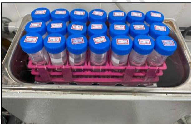
Fig.2. Polyethylene bottles with coupons on thermostatic bath
