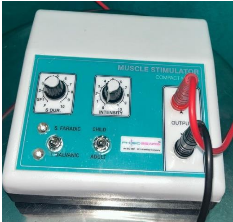
FIGURE 4: Galvanic And Faradic Muscle Stimulation Equipment.
